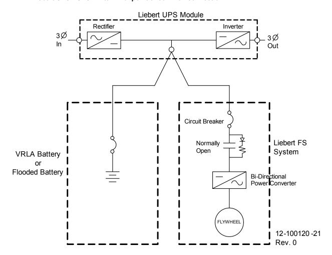
Figure 143One-line diagram, single Liebert FS and battery with factory-integrated circuit breaker supplying Liebert UPS—UPS battery point of common connection
